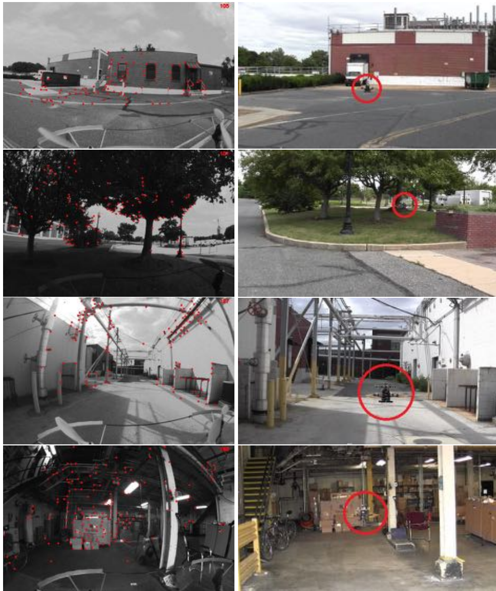
Figure 5.6: Images from the onboard camera (left column) and corresponding images from an external camera (right column). Note the vast variety of environments, including open space, trees, complex building structures, and indoor environments. We highlight the position of the MAV with a red circle.
