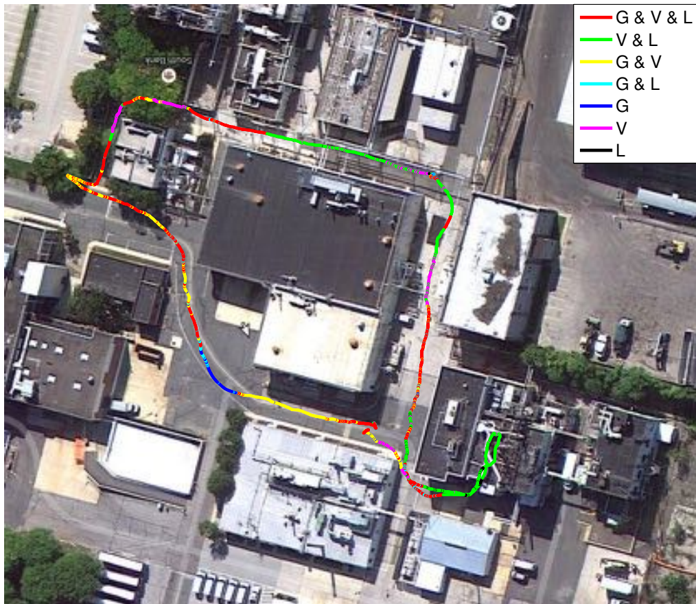
Figure 5.7: Vehicle trajectory aligned with satellite imagery. Different colors indicate different combinations of sensing modalities. G=GPS, V=Vision, and L=Laser.
