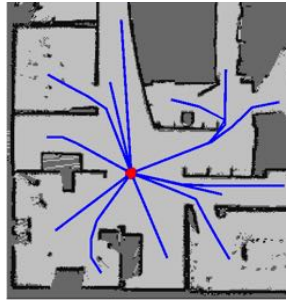
Figure 4.2: Representative actions generated by path planning. Blue lines show shortest paths from the red circle to nearby locations using an occupancy grid.
