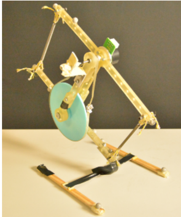
Figure 3.1: Illustration of the segmented beam hopper. Its model consists of 3 rigid bodies, two linear springs, one torsional spring, and is driven by a sinusoidal input torque.
