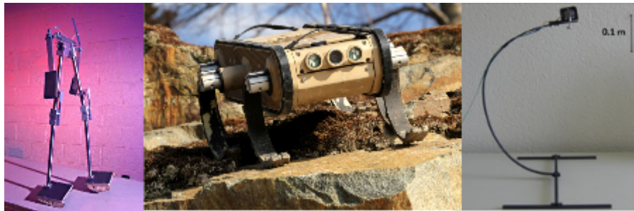
Figure 1.3: Illustration of various feedforward controlled robots. From left to right: Passive dynamic walker 1 , RHex 2 , Curved beam hopper 3 .
