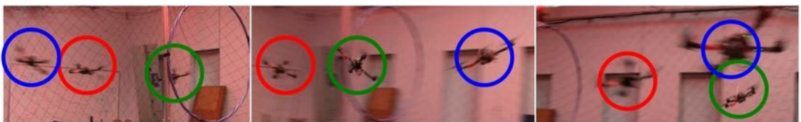
Figure 7.4: Snapshots of the three quadrotor experiment in which the hoop represents the gap. See the attached video or http://tinyurl.com/multiquad .
