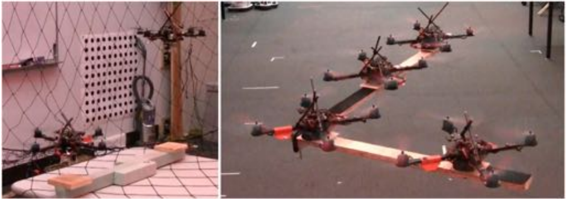
Figure 3.4: Left: Image from an experiment with the gripping mechanism enabling cooperative grasping, manipulation, and transportation. Right: Four quadrotors carrying a payload in the El configuration. Videos of the experiments are available at http://tinyurl.com/pennndars .
