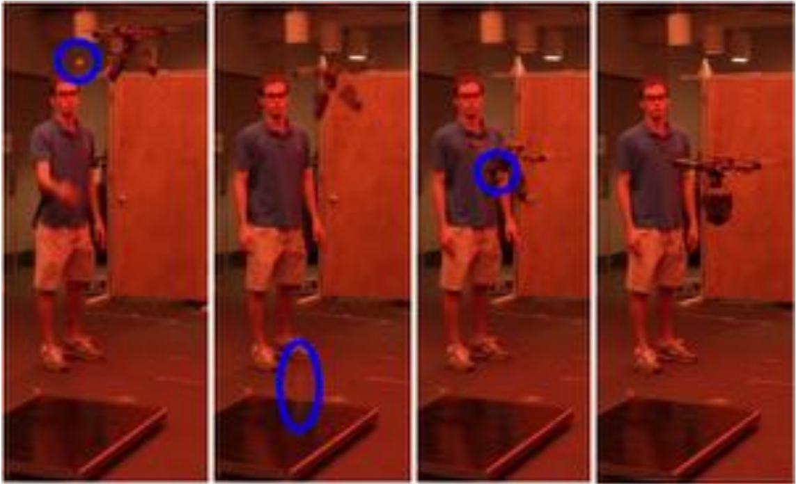
Figure 6.9: Quadrotor catching a thrown ball after a bounce. The ball is highlighted in blue.
