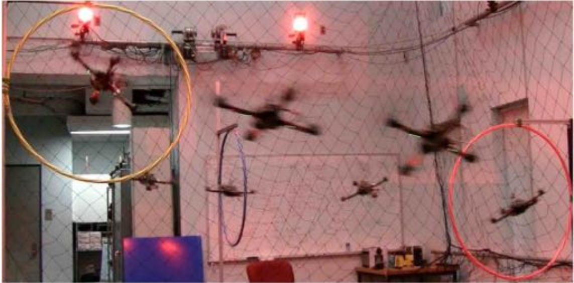
Figure 6.4: Composite image of a single quadrotor quickly flying through three static circular hoops. See attached video or http://tinyurl.com/pennquad .
