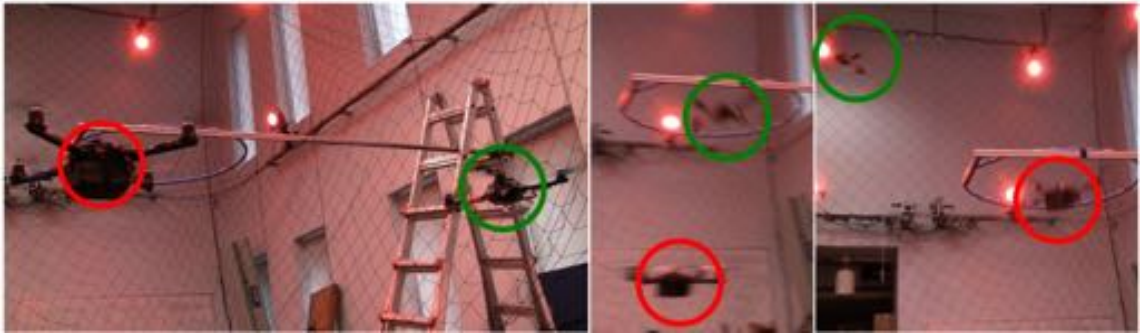
Figure 7.6: Snapshots of an experiment with the kQuad1000 (quadrotor 1, red) and the AscTec Hummingbird (quadrotor 2, green) in which the hoop represents the horizontal gap. See the attached video or http://tinyurl.com/multiquad .
