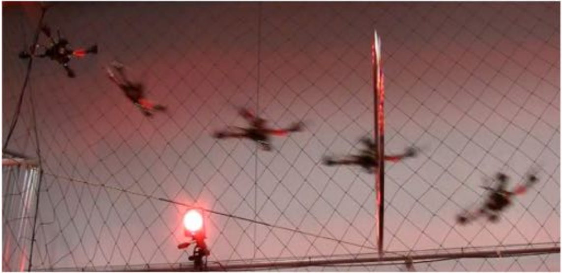
Figure 6.6: Composite image of a single quadrotor flying through a thrown circular hoop. See attached video or http://tinyurl.com/pennquad .
