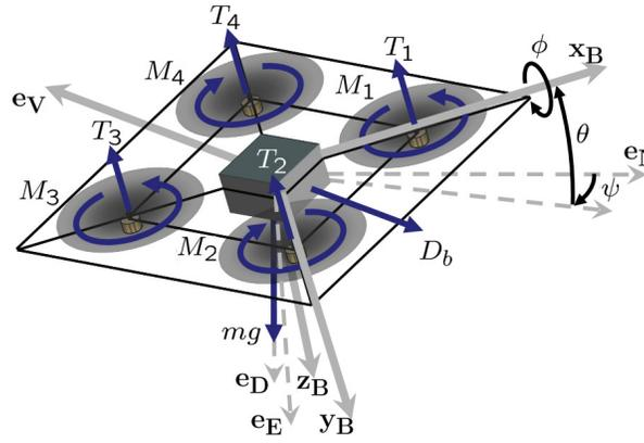
Figure 2. Free body diagram of a quadrotor helicopter. The roll, pitch and yaw angles are denoted  $\phi$ ,  $\theta$ , and  $\psi$ , respectively. Motors are labeled 1 – 4, with thrust  $T_i$  and moments  $M_i$ . The force due to gravity,  $mg$ , acts in the downward direction and drag forces  $D_b$  act opposite the direction of the free stream velocity  $e_v$ .
