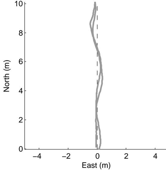
Figure 7. Tracking a trajectory outdoors, at 2.0 m/s, with an error of under 0.5 m. GPS is used for position, and nominal winds were measured at 5-10 mph.
