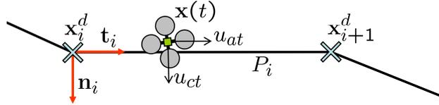
Figure 5. Vehicle path definition. While the quadrotor travels along segment  $P_i$  from waypoint  $\mathbf{x}_i^d$  to  $\mathbf{x}_{i+1}^d$ , it applies along track and cross track control inputs  $u_{at}$  and  $u_{ct}$  to follow the path segment.
